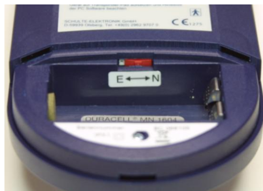
Fig.4: Sensitivity switch of the respiration channel in the battery compartment.
