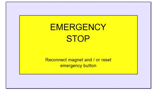
When an emergency stop is made on a treadmill this screen becomes visible. The belt will stop and the elevation will remain as it is at that time.
