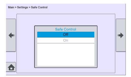
In case you would not like to allow the subject to unexpectedly operate the treadmill (e.g. a child) you can set up "Safe Control". In this case the setting of speed and elevation can not be done with 1 hand.
