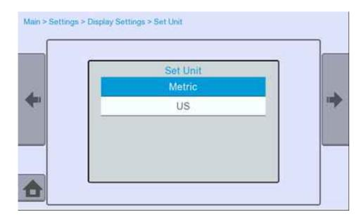
The Control Unit can display the parameters in Metric or US.
